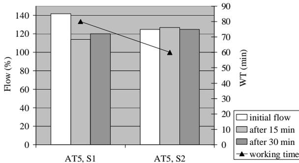
Figure III: Flow profile and working time for castable AT5
