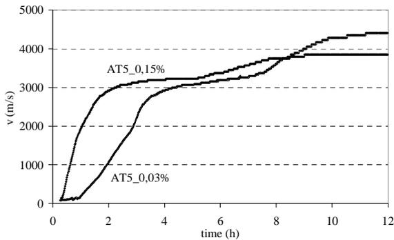
Figure V: Velocity for AT5 castable with different phosphate contents
