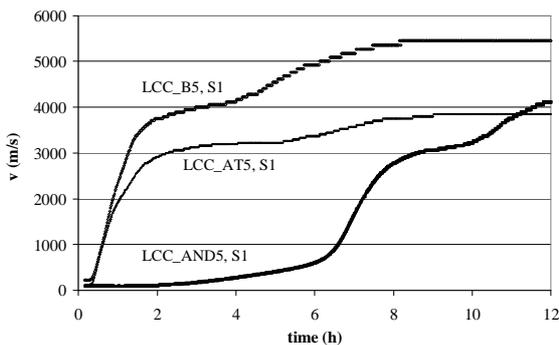
Figure VI: Velocity for the different castables (S1)
