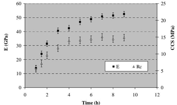
Figure IV: Evolution of strength and elastic modulus over the time for castable AT5\_S2
