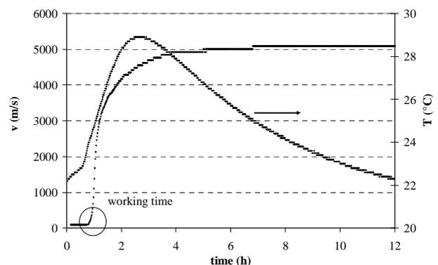
Figure II: Velocity and exothermic profile for castable AT5, S2
