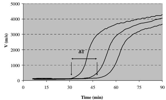
Figure VII: Example of variations in the ultrasonic velocity curve due to external parameters (castable AT5\_S2)
